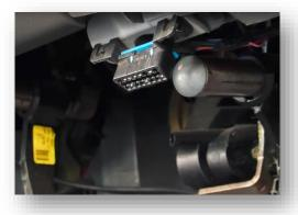
Step 2 Connect the OBD end of the ROVR (A1) into the vehicle's OBD port (A2)
